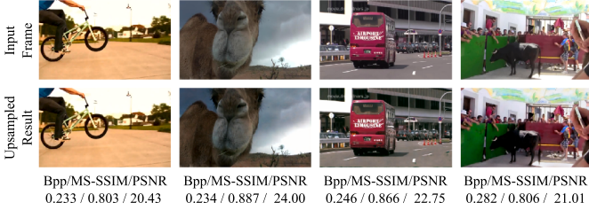
Fig. 15. Visualization of the upsampled results. The “up-then-down” branch can coarsely reconstruct the original content in the pixel domain, which helps the feature transfer process gain knowledge of pixel-domain content.
