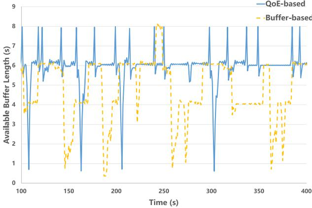
Fig. 8. Comparison of the available buffer length between “QoE-based” and “Buffer-based”.
