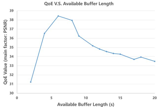
Fig. 13. QoE performance under different available buffer length settings.
