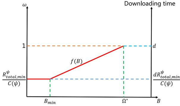
Fig. 6.  $\omega$  selection as a function of buffer occupancy.
