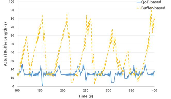
Fig. 9. Comparison of the actual buffer length between “QoE-based” and “Buffer-based”.
