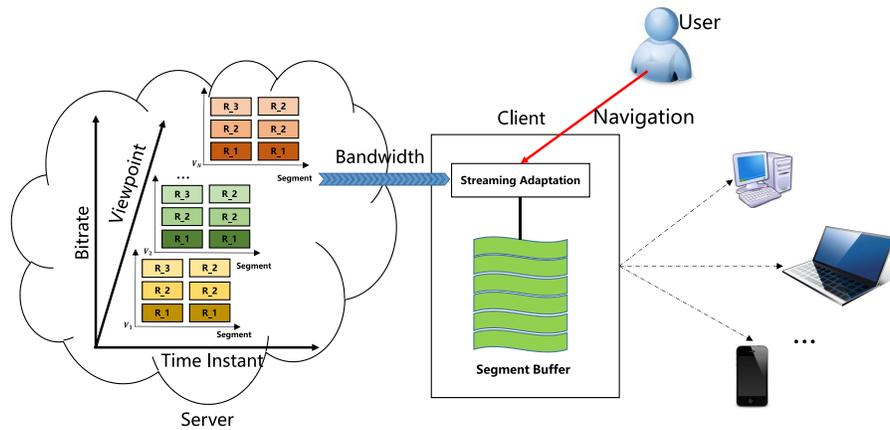
Fig. 1. The diagram of multiview video streaming over DASH. During the streaming process, the client is able to switch among different viewpoints as well as different representations.
