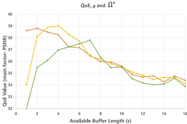
Fig. 15. QoE, Ideal buffer length with different  $\mu$ , where red line is with  $\mu = 50$ , yellow line is with  $\mu = 100$ , and green line is with  $\mu = 300$ .
