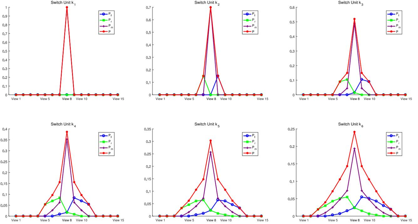
Fig. 4. Estimated probability of each view in 6 switch units,  $p_1 = 0.7$ ,  $p_2 = 0.6$  and  $p_3 = 0.3$ : in the sub-figure, the horizontal axis denotes viewpoints, where the central view is View 8, the vertical axis represents the switch probability.
