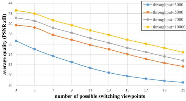
Fig. 5. How  $\bar{Q}$  changes with the number of the possible switching viewpoints in different network condition.
