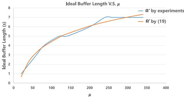
Fig. 14. Ideal buffer length  $\Omega^*$  with different  $\mu$ : the blue line represent the actual settings of  $\Omega^*$  corresponding to  $\mu$ , and the red line is calculated as (19).
