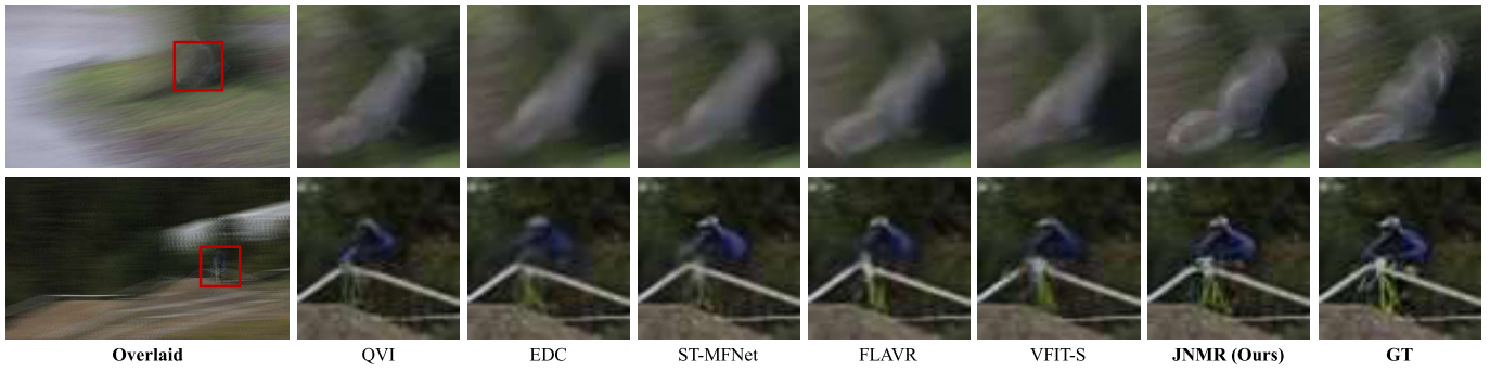
Fig. 8. Qualitative comparisons against the state-of-the-art multi-reference interpolation algorithms with the Vimeo-90K Septuplet dataset. The middle frames generated by JNMR have clear high-frequency structures and few artifacts compared with other models when dealing with large and complicated motions.
